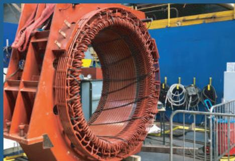
Stator Asynchrone – 3000 kW – 6600V – 300tr/min
